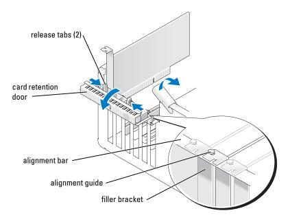
Push the two release tabs on the card retention door from the inside to pivot the door open. Because the door is captive, it will remain in the open position.
